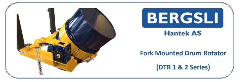
Fork Mounted Drum Rotators are designed for manual rotation of 210 litre drums. The attachment simply slides onto the truck forks, thus allowing 360 degree controlled pouring/rotation via the gearbox. Variations of models allows for either crank handle rotation or loop chain rotation
