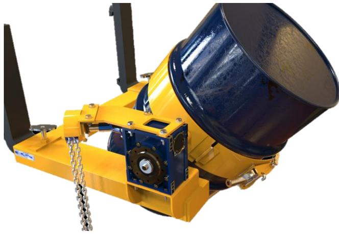
Fork Mounted Drum Rotators are designed for manual rotation of 210 litre drums. The attachment simply slides onto the truck forks, thus allowing 360 degree controlled pouring/rotation via the gearbox. Variations of models allows for either crank handle rotation or loop chain rotation
