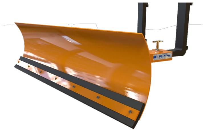
Fork Mounted Snow Ploughs offer a fixed blade position which clears the snow to the right. The bottom of the blade on the snow plough is protected by a rubber blade insert.
